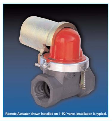
The Model 501 Remote Actuator will add an additional layer of protection to panic switches, fire and sprinkler alarm systems. A CALIFORNIA valve with the 501 Remote Actuator will trip during a violent earthquake or when an electrical signal is present.
