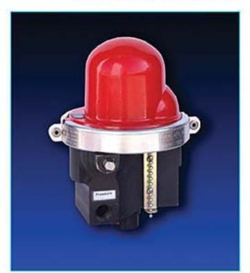
The Model 400 earthquake actuated 3 way valve offers a redirection of dry air or nitrogen from the pressure ( n/o ) to the exhaust ( n/c ) port during a seismic event. Reset is simple using a flat blade screw driver and the valve status window, see included instructions.
